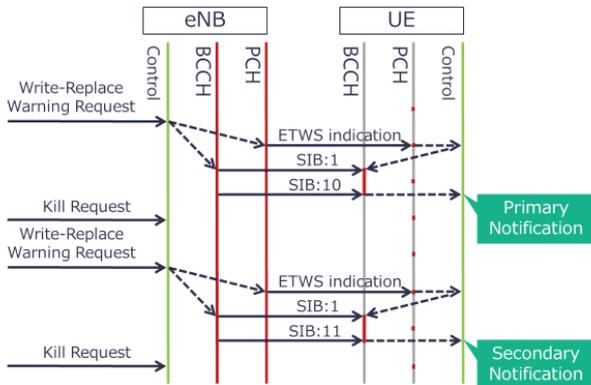
Fig. 3. Sequence for delivering an emergency bulletin by ETWS
