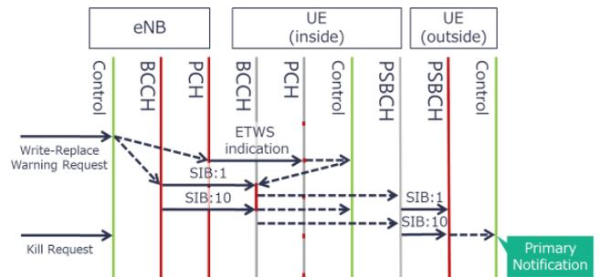
Fig. 5. Sequence for delivering an emergency bulletin
