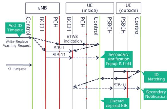
Fig. 7. Sequence for delivering emergency bulletins by the proposed system
